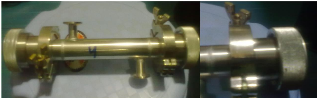
Figure-2: Resonance cavity with filter( Length= 27cm & Radius =1.4cm (with a filter))
